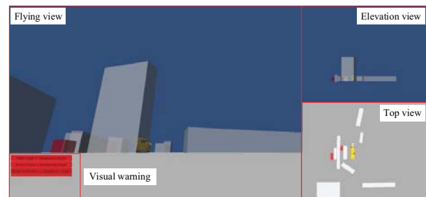
Figure 3: User interface of the on-board display and warning system
